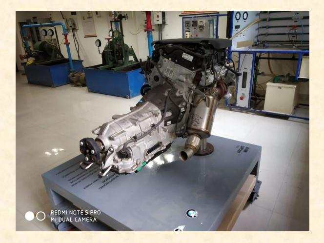
Twin Power Turbo, Inline 4 cylinder diesel engine
