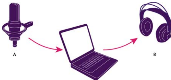
A Sound card inputs connect to sources such as microphones and tape decks. B Sound card outputs connect to speakers and headphones.
