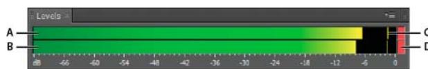
Levels panel, docked horizontally A Left channel B Right channel C Peak indicators D Clip indicators
